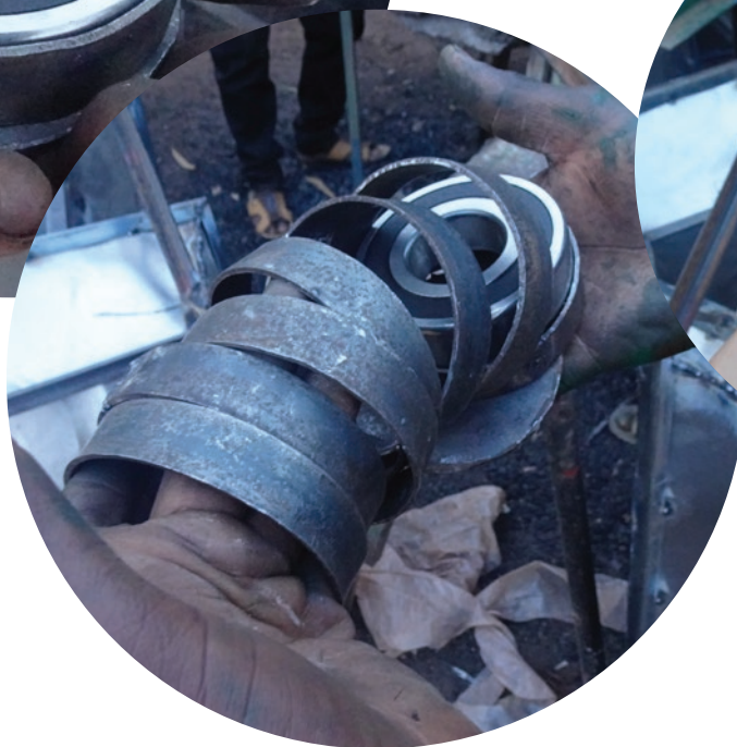
roller bearing box assembling manual cutting of metal plates
